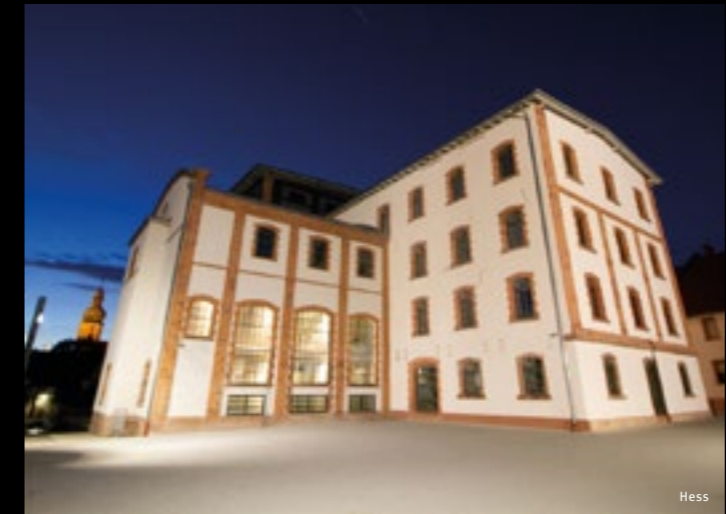
The dark windows are the proof that the surfaces are exactly blocked by the projection technology – and therefore a blinding of persons in the building is avoided.
